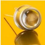
Concentrating lens creating a virtual active area of 55 * real active area. This approximately multiplies the current by factor 55 while using the same chip active area. A disadvantage is a strongly reduced field of view compared with the flat window type. |
